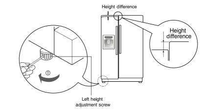
Level the door by inserting flat ( - type) driver into the groove of the right height adjusting screw and rotate it clockwise  $(\mathbb{O})$ .
